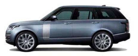
Standard Wheelbase (SWB) 2.922mm Long Wheelbase (LWB) 3.122mm
