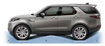
Approach Angle Ride Height 34.0° Air suspension Coil suspension 26,3°
