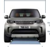
Height suspension 1.888mm Coil suspension 1.909mm
